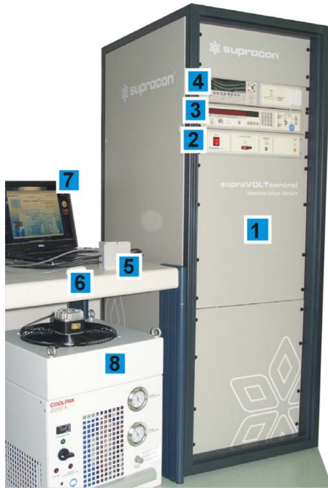
Fig. 1. Photograph of the cryocooler-based Josephson voltage standard system “supraVOLTcontrol” including the following components: 1: Pulse tube cooler with a SIS Josephson junction array and the 75 GHz microwave electronics installed in the 19” rack, 2: Control electronics, 3: EIP 578B source locking counter, 4: Keithley 2182A nanovoltmeter, 5: 3-channel polarity reversal switch, 6: Sensors for temperature, pressure and humidity, 7: Laptop, 8: compressor unit with an input power of 2.5 kW.
